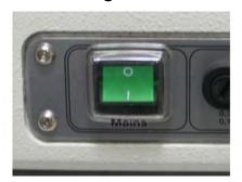
Switch main switch to I. The rotary cone sample divider starts up.
